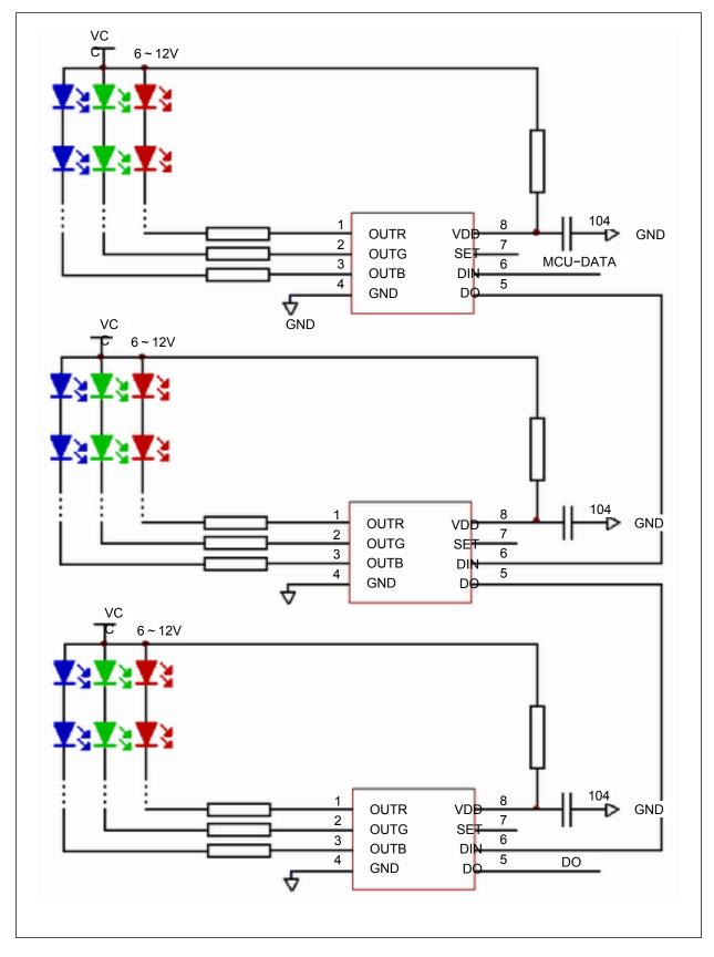
The power supply voltage for the UCS1903 may be selected from 6V to 12V. A 104 capacitor between the power supply and the ground should be connected as close to the UCS1903 package as possible, and the PCB traces should be as short as possible. A resistor R should be connected between the power supply and the VDD pin, with the resistance value determined in reference to the supply voltage. The recommended resistance value is as follows:
