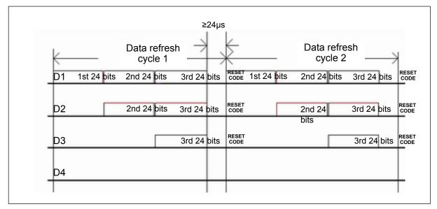
**Note:** D1 is the data sent from the MCU, D2, D3 and D4 are the data automatically shaped and forwarded by the cascaded circuit.
